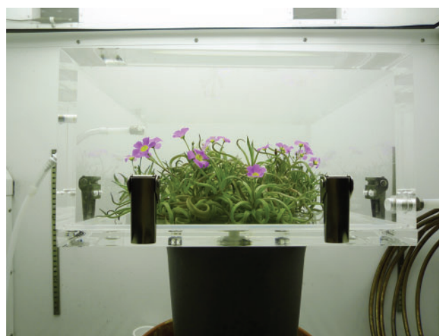
Fig. 1. A flowering Calandrinia polyandra growing inside a Perspex CO 2 exchange cuvette in a growth chamber. The roots and pot are outside the cuvette but inside the chamber. Cuvette internal width = 30 cm.
